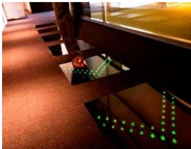
Fig 6 - Power-Generating Floor™ tiles at the Kokuyo headquarters.
