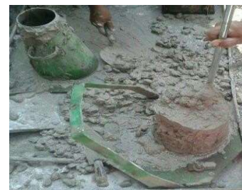
Fig. Testing of slump cone
