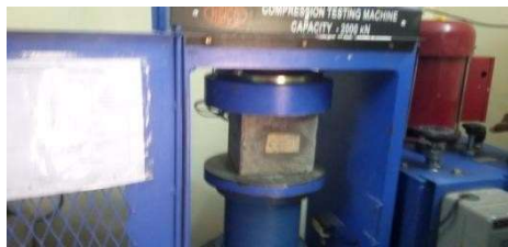
Fig. view of testing cube
