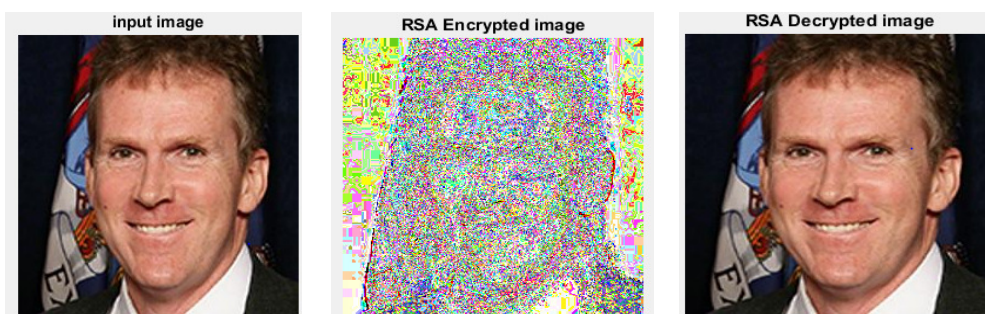
Fig. 4: Example of RSA encryption and decryption; p=13 , q=31 , n=403 , \phi=360 , e=7 , d=103
